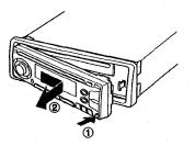
Do NOT touch the connector on the reverse side of the front panel, as doing so may contaminate the connector and cause a poor connection resulting in a malfunction. Attaching the front panel
